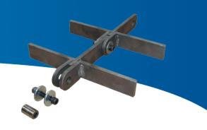
VO chain consists of welded sheet steel in fork-shaped links. The links are easy to assemble and disassemble using a pin and Allen bolt. The chain is fitted with welded-on scrapers made of folded material. Standard chain widths are 260, 360, 460, and 560 mm. Intermediate sizes are available.
